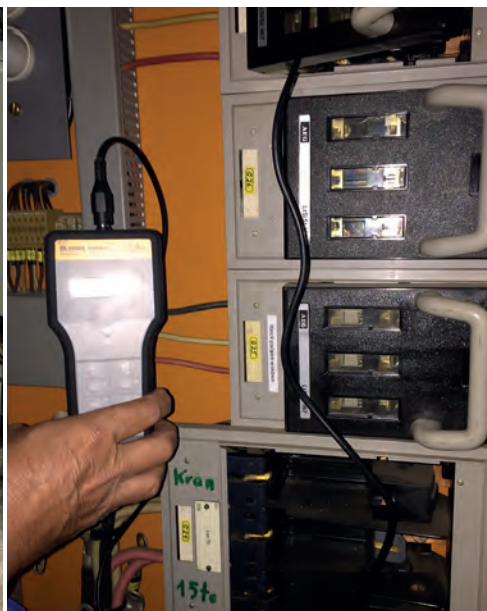
Fault location with the portable insulation fault locator EDS195P
