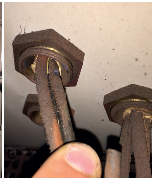
This was where the phase lay on the housing, causing the insulation fault
