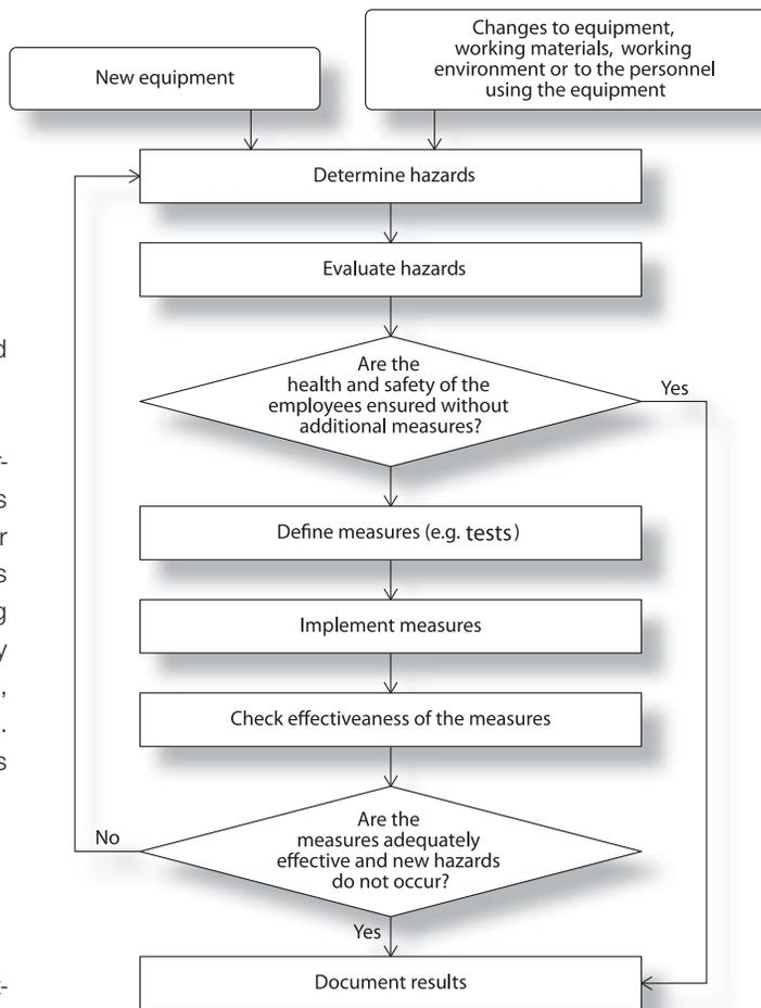
Fig. 1 Basic process for determining and assessing hazards as well as for deriving of measures. (Fig. 1 in TRBS1111, [1,2])
