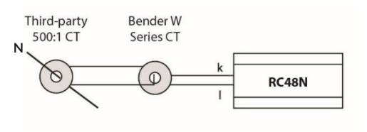
Fig 3: Cascaded CT connection example
