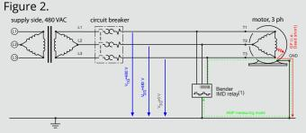
Figure 2: Ungrounded three-phase system with IMD
