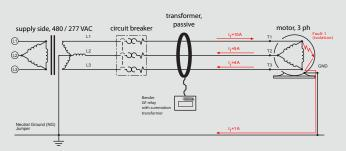
Figure 5: Faulted three-phase grounded system with zero-sequence relay
