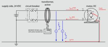
Figure 6: Grounded DC power system
