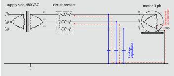
Figure 1: Ungrounded system in single-fault condition
