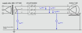
Figure 4: Simplified wye-configured, 480/277 V three-phase system
