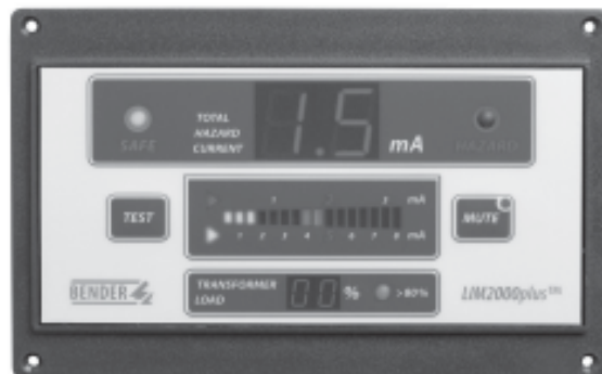
Line Isolation Monitor LIM2000plus™
