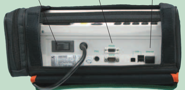
ON/OFF switch Multi-functional interfaces PS/2, USB, RS-232, RS-485 Ethernet
